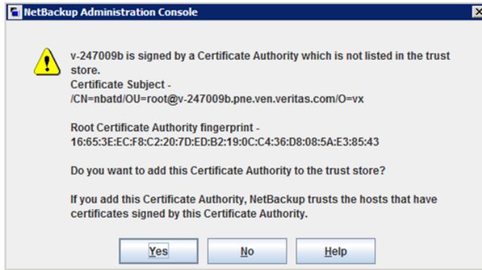
Figure 15-1 Message inquiring whether to add a Certificate Authority (CA) to the trust store
