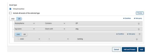
This example uses **AND** to narrow the scope of the query: It selects only the VMs that have cp in their display name and that also have a tag name as eng, and are in running state.
