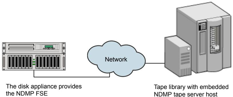
**Figure 2-4** Separate host provides NDMP tape server functionality
