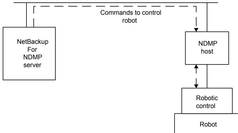
The following figure shows how the robot is controlled in the same way as the other robots on NetBackup servers.
