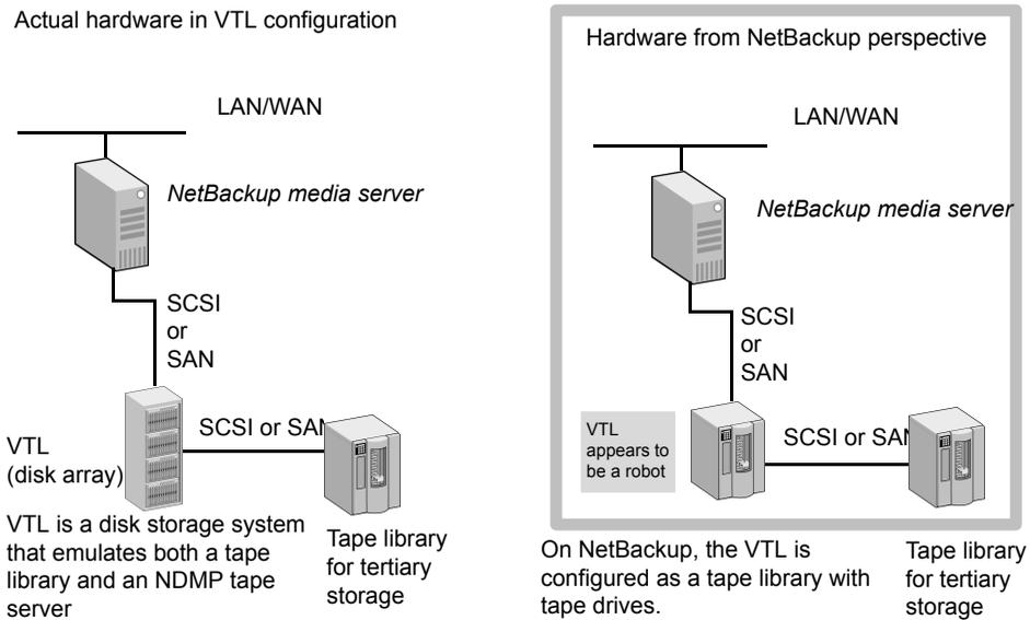
The following figure shows the data flow and control for a VTL.
