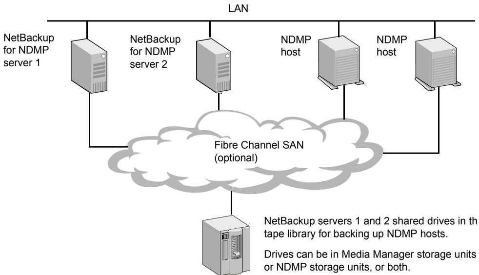
For each robot, either a NetBackup media server or an NDMP server (not both) can handle robotic control.
