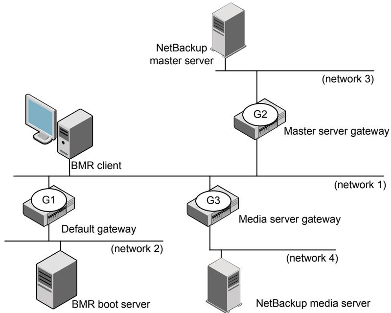
The client in this diagram cannot communicate with all of the servers it needs to by using only the default gateway. For such a configuration, you should specify the default gateway as G1, the master server gateway as G2, and the media server gateway as G3.
