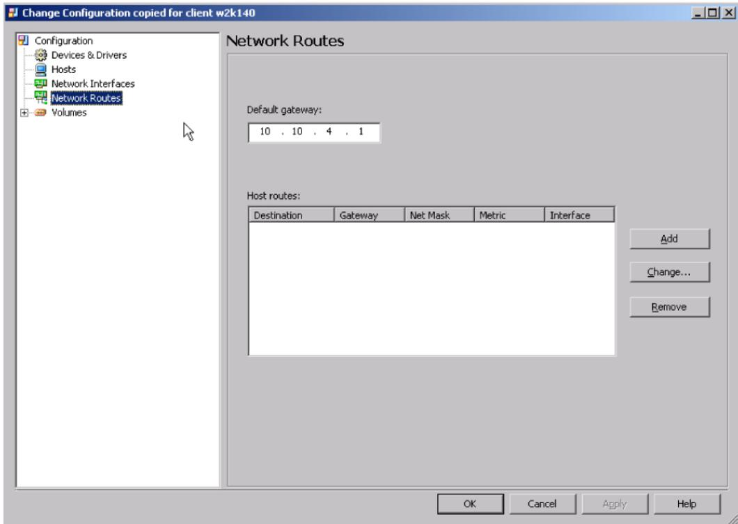
You may need to add a route if an existing route in the configuration is not sufficient to reach the NetBackup or BMR servers. This situation can occur during disaster recovery at a different location when you move servers from one subnet to another. It also can occur when any routers that intervene are changed.
