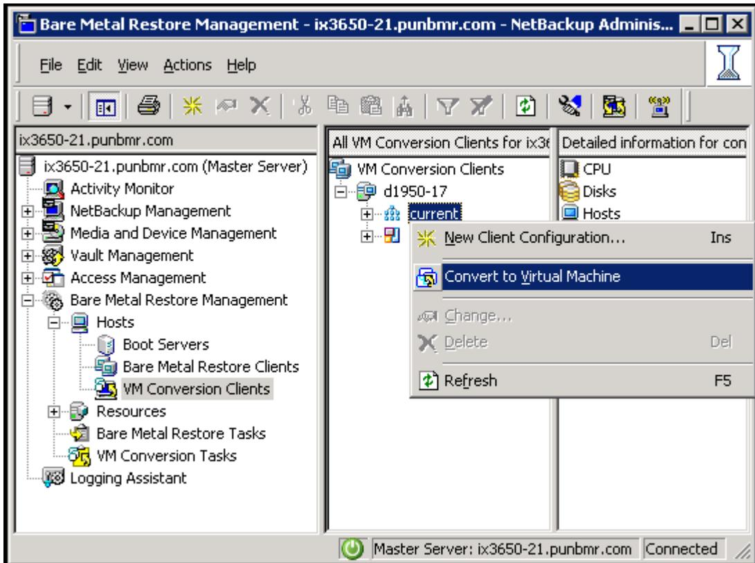
Optionally, you can create a custom client configuration or PIT (Point-In-Time) configuration for VM creation. In such case, use **New Client Configuration** option to either create a PIT configuration or copy the existing client configuration. For details on how to change client configuration, See [“Creating custom configurations”](#) on page 243.
