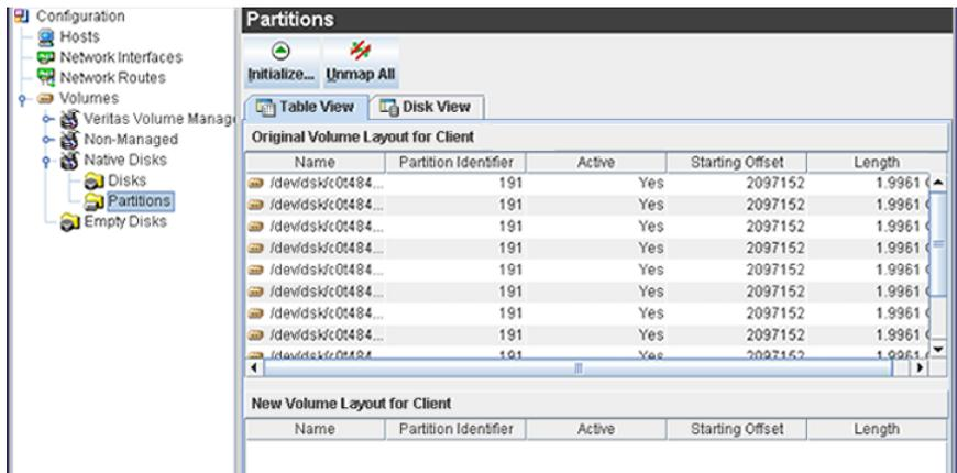
You can map the partition by using the mapping wizard. Right-click the Volume to launch the mapping wizard. You can map the source partition to destination disk and specify the percentage space of the destination disk to use for creating the partition.
