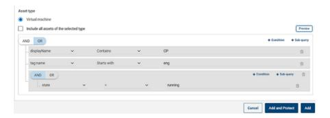
This example uses **AND** to narrow the scope of the guery: It selects only the VMs that have cp in their display name and that also have a tag name as eng, and are in running state.
