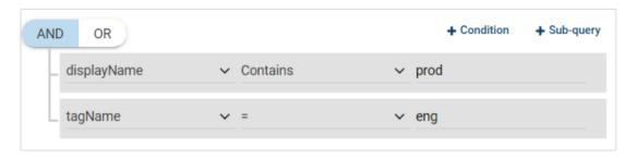
This example uses **AND** to narrow the scope of the guery: it selects only the VMs that have prod in their display name and that also have a tag named eng. If a VM does not have prod in its display name as well as a tag named eng, that VM is not added to the group.
