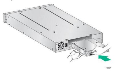
4. To secure the tape drive to the chassis, use a torque driver to tighten the thumbscrews on the drive sled to 6 inch pounds or 0.68 N m.
