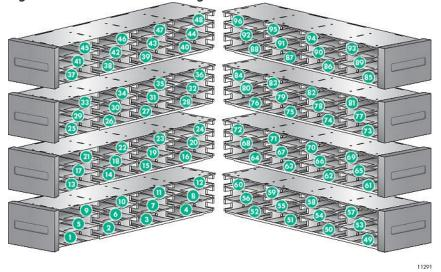
When the MSL8096 lower-left mailslot or the MSL8048 mailslot is enabled, all of the storage slot numbers are adjusted. The storage slots in the other magazines are renumbered accordingly.
