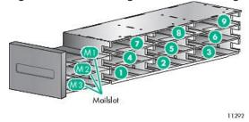
On the MSL8096, when the upper-right mailslot is enabled, the numbering of the storage slots in the other magazines is not affected. When both mailslots are enabled, the mailslot numbers in the upper-right magazine are adjusted, as shown in the following illustration.
