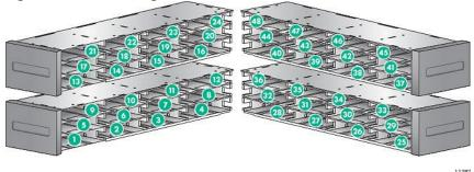
When the mailslot is enabled, all of the storage slot numbers are adjusted. The storage slots in the other magazines are renumbered accordingly.
