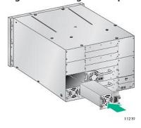
3. Tighten the blue thumbscrews to secure the power supply to the library.
