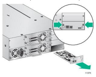
4. Position the new library controller on the alignment rails and slide it into the library until it is flush with the back panel. Tighten the two blue thumbscrews to secure the card to the library.
