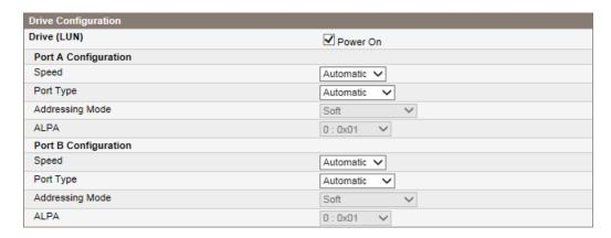
For a Fibre Channel tape drive, you can use this screen to configure the FC ports. The port fields are:
