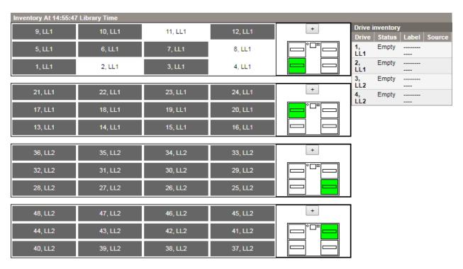
A dark rectangle indicates a full slot, a red rectangle indicates a cartridge with a problem, and a white rectangle indicates an empty slot.
