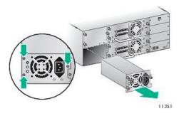
3. Position the new power supply on the alignment rails and slide it into the library until it is flush with the back panel. Tighten the three blue thumbscrews to secure the power supply.
