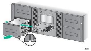
4. On the MSL8096, the magazine in the upper right side will be unlocked if it is configured as a mailslot and you choose to open it. To open the upper right magazine, grasp the magazine and pull it straight out until you can access the desired slot.
