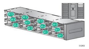
Figure 5. MSL8096 upper-right magazine slot numbering with both mailslots enabled
