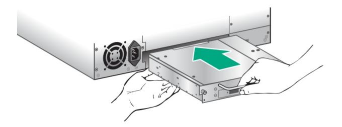
4. To secure the tape drive to the chassis, use a torque driver to tighten the thumbscrews on the drive sled to 6 inch pounds or 0.68 N m.
