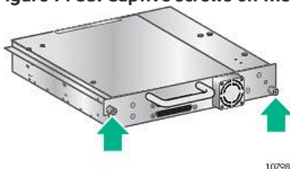
Figure 7785: Captive screws on the tape drive
