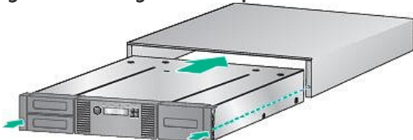
Figure 4: Installing the tabletop conversion cover
