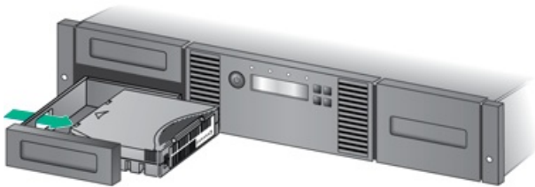
Figure 51: Removing a tape from the mailslot
