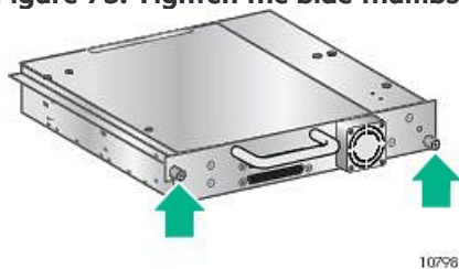
Figure 75: Tighten the blue thumbscrews
