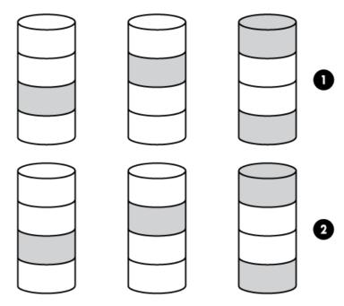
For any given number of drives, data loss is least likely to occur when the drives are arranged into the configuration that has the largest possible number of parity groups. For example, four parity groups of three drives are more secure than three parity groups of four drives. However, less data can be stored on the array with the larger number of parity groups.
