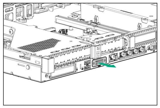
8. Connect the serial cable option, and then secure the cable with two T-10 screws. Then, remove the backing from the double-sided tape and press down where indicated.
