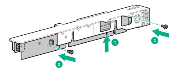
10. Install the drive cage on the riser cage.
