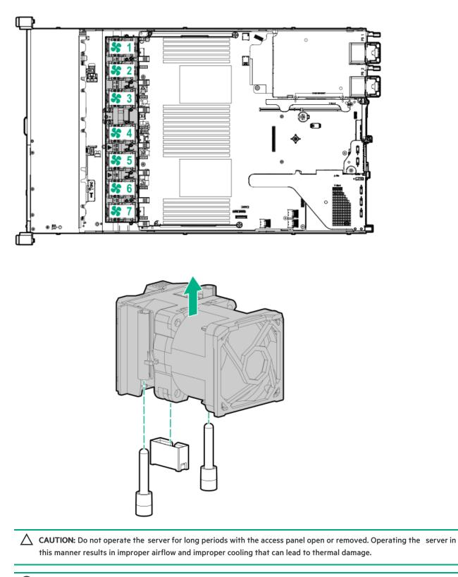
(i) IMPORTANT: For optimum cooling, install fans in all primary fan locations.
