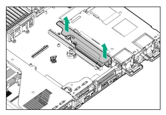
8. Lift and remove the secondary riser cage latch.
