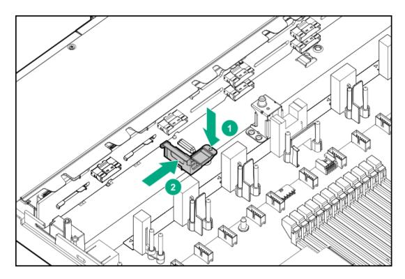
6. Slide the energy pack into the left retainer, and then install the right retainer.
