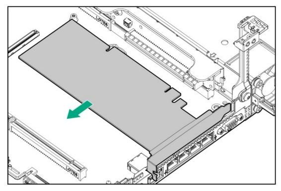
10. Remove the PCI riser cage.
