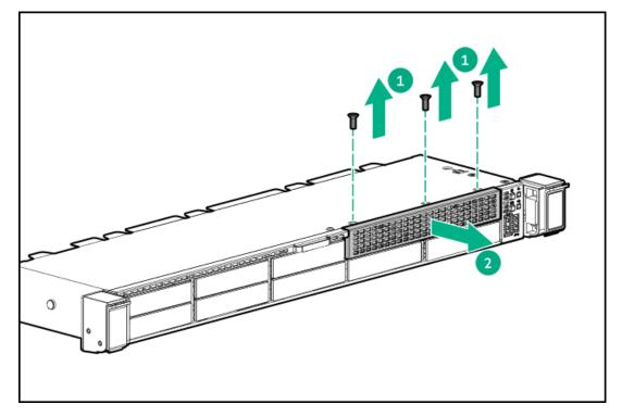
7. Install the 8 SFF display port/USB/optical blank option.
