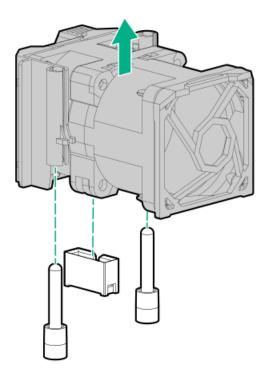
7. Remove fan blanks from the fan bays, if installed.
