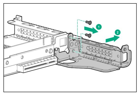
7. If installed, remove the low-profile riser cage.
