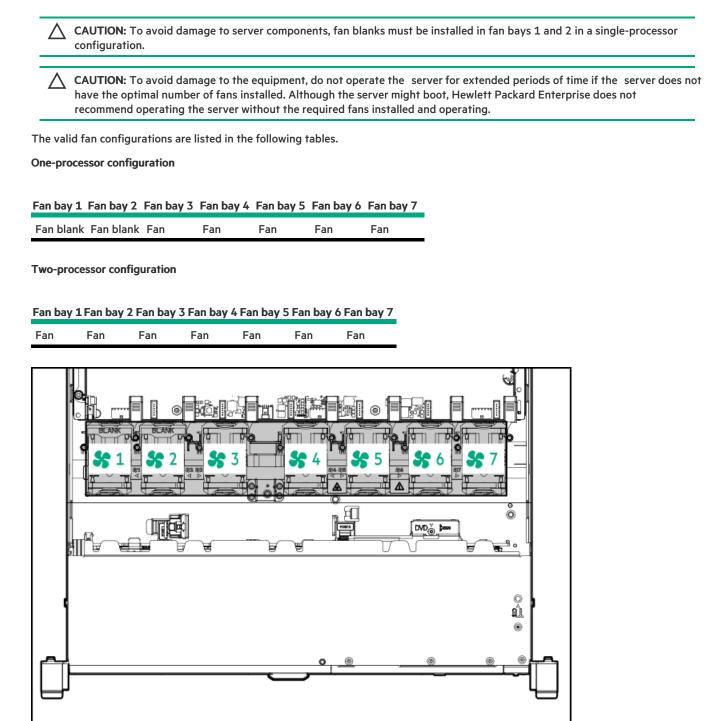
The loss of a single fan rotor (one standard fan) causes loss of redundancy. The loss of two fan rotors (two standard fans or one high performance fan) causes the server to initiate a shutdown.
