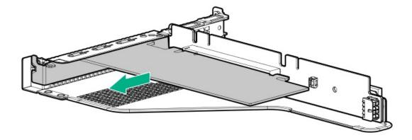
8. Remove the existing riser board from the PCI riser cage.
