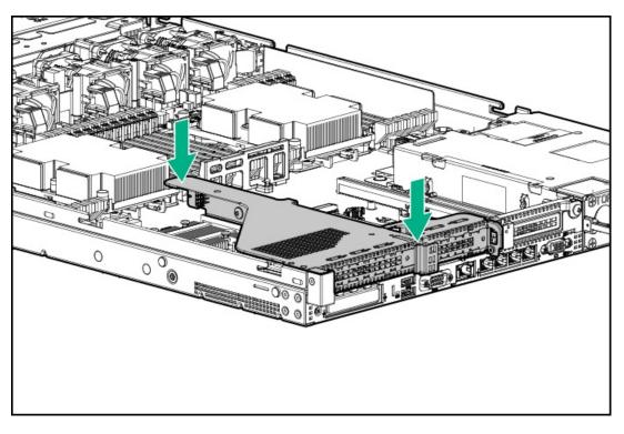
15. Apply the label that reads, "Card with cable attached. Remove riser with care" to the top of the PCIe riser cage.
