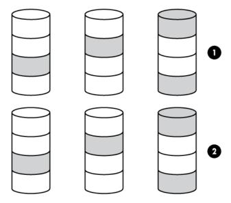
For any given number of drives, data loss is least likely to occur when the drives are arranged into the configuration that has the largest possible number of parity groups. For example, four parity groups of three drives are more secure than three parity groups of four drives. However, less data can be stored on the array with the larger number of parity groups.
