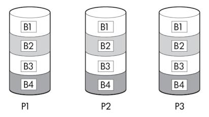
When the array has more than six physical drives, drives are mirrored in trios, and the fault-tolerance method is known as RAID 10 Triple. If a physical drive fails, the remaining two drives in the mirrored trio can still provide all the necessary data. Several drives in the array can fail without incurring data loss, as long as no three failed drives belong to the same mirrored trio. The total drive count must increment by 3 drives.
