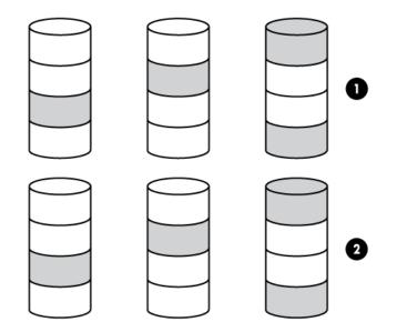
For any given number of drives, data loss is least likely to occur when the drives are arranged into the configuration that has the largest possible number of parity groups. For example, four parity groups of three drives are more secure than three parity groups of four drives. However, less data can be stored on the array with the larger number of parity groups.
