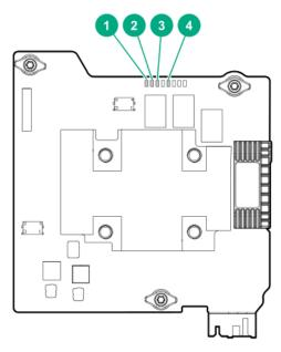
Immediately after you power up the server, the controller runtime LEDs illuminate briefly in a predetermined pattern as part of the POST sequence. At all other times during server operation, the illumination pattern of the runtime LEDs indicates the status of the controller.
