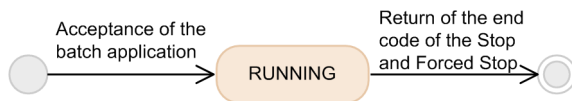
Figure 2–8: State transition of a batch application (When the scheduling functionality is not used)
