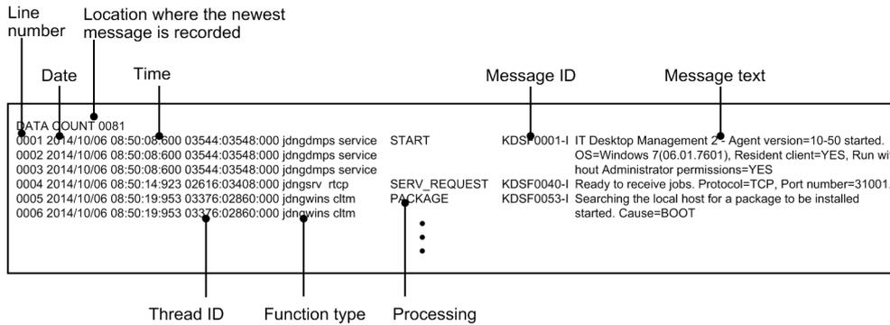
In the USER\_CLT.LOG file, the number of the line on which the newest message is recorded is output to the first line. Messages are output to the second and following lines. You can track the operations of Agent from the date, time, message ID, or message text of each message. On the second and following lines, fixed items are output at fixed positions (columns). The following shows the location of each item:
