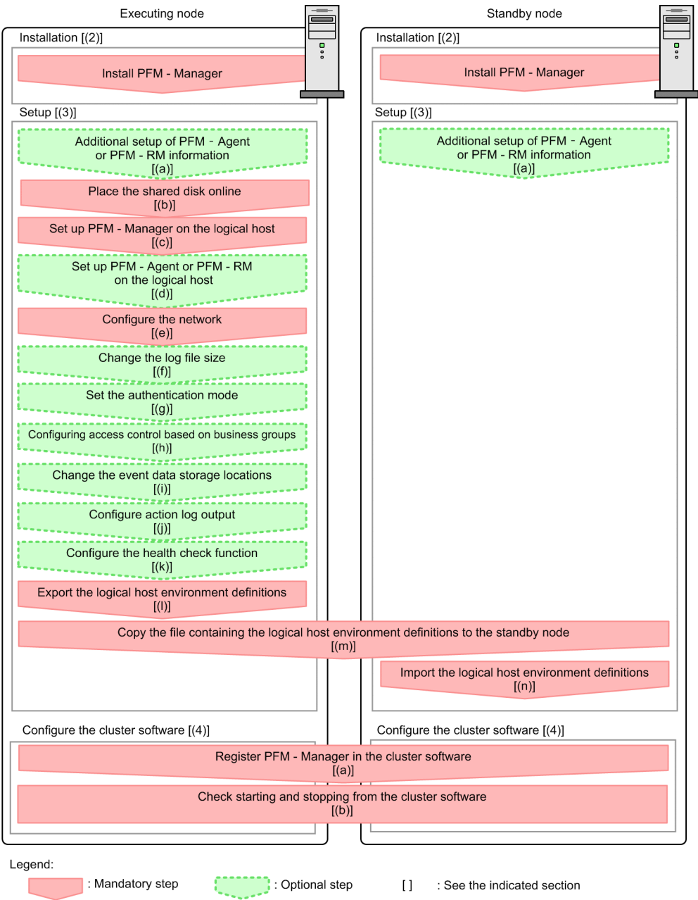
Figure 10–10: Process flow for installation and setup of PFM - Manager used on a logical host (in Windows)
