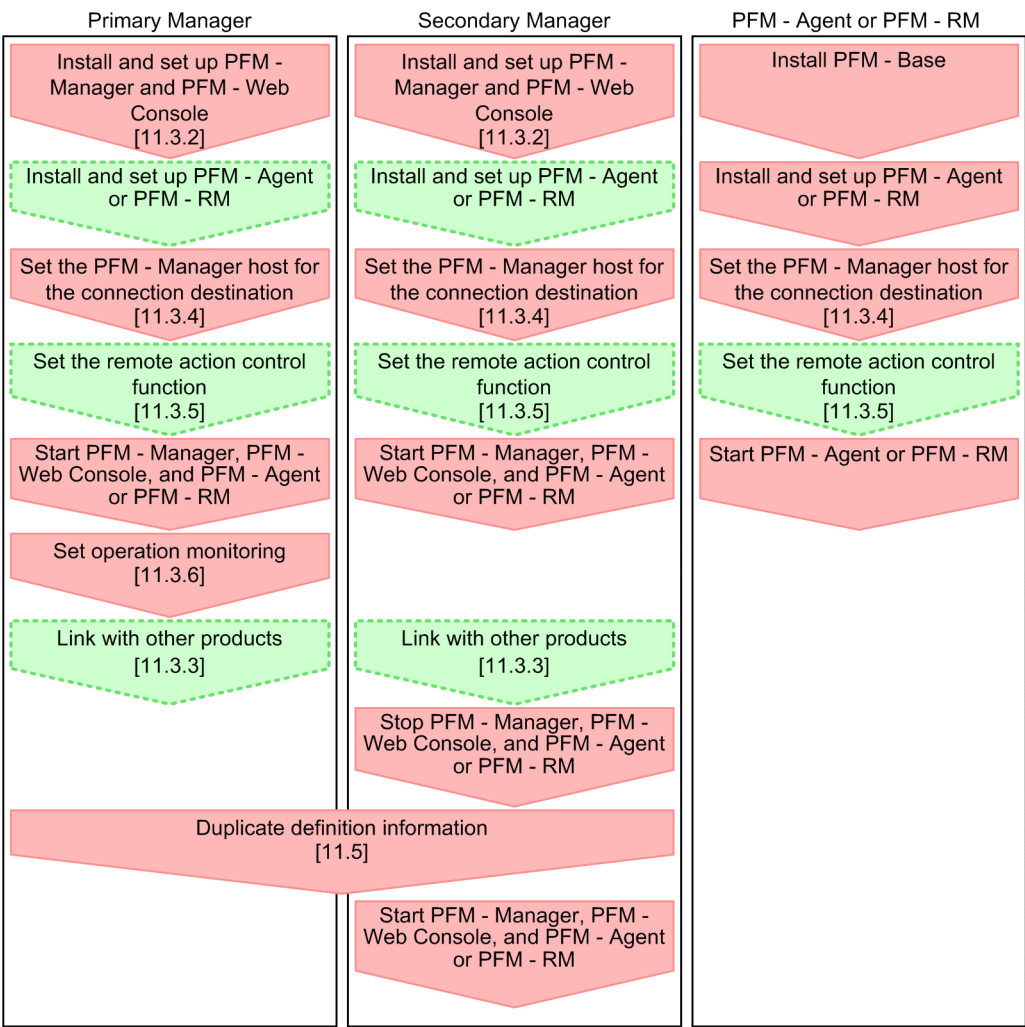
Figure 11–4: Setup procedure when the primary Manager and the secondary Manager are newly installed
