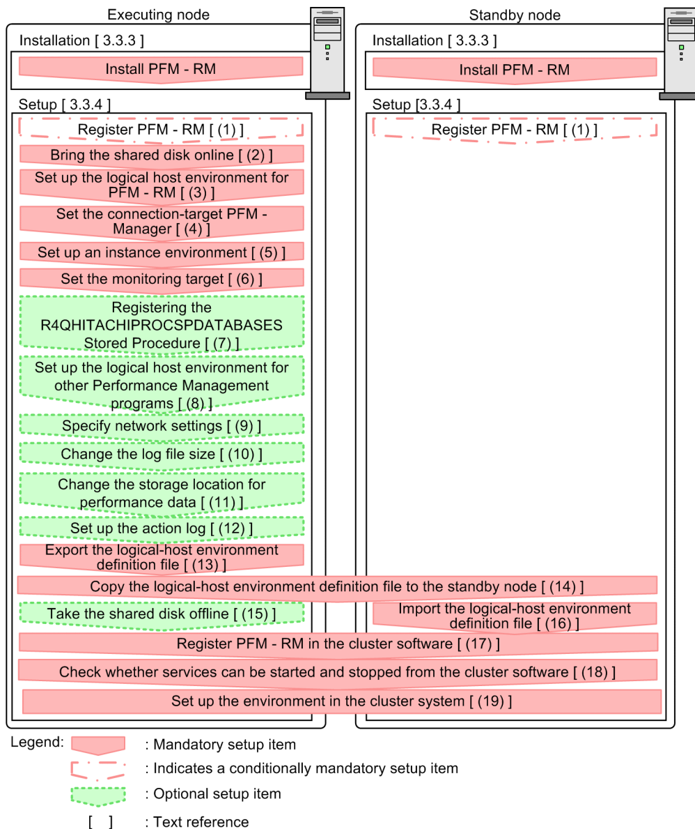
Figure 3–6: Workflow for installing and setting up PFM - RM for Microsoft SQL Server to run on a logical host in a cluster system
