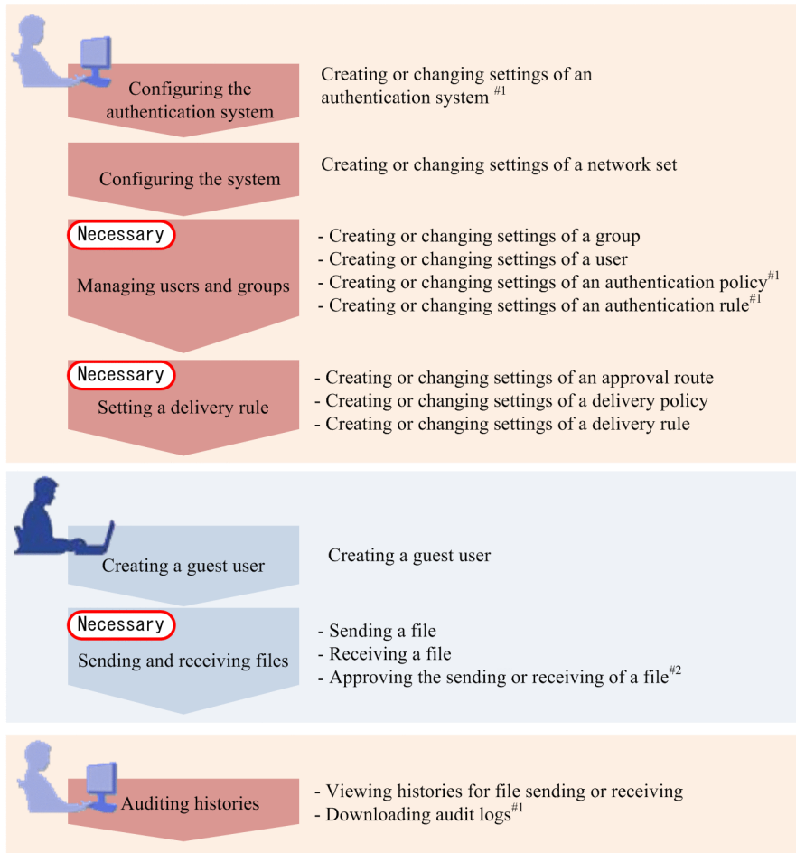
Figure 2–1: General operation procedure for JP1/DH - Server
