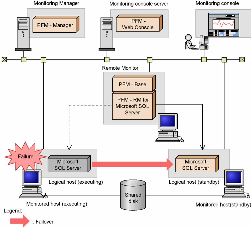
Figure 1-2: Example of an PFM - RM for Microsoft SQL Server configuration in an HA cluster system
