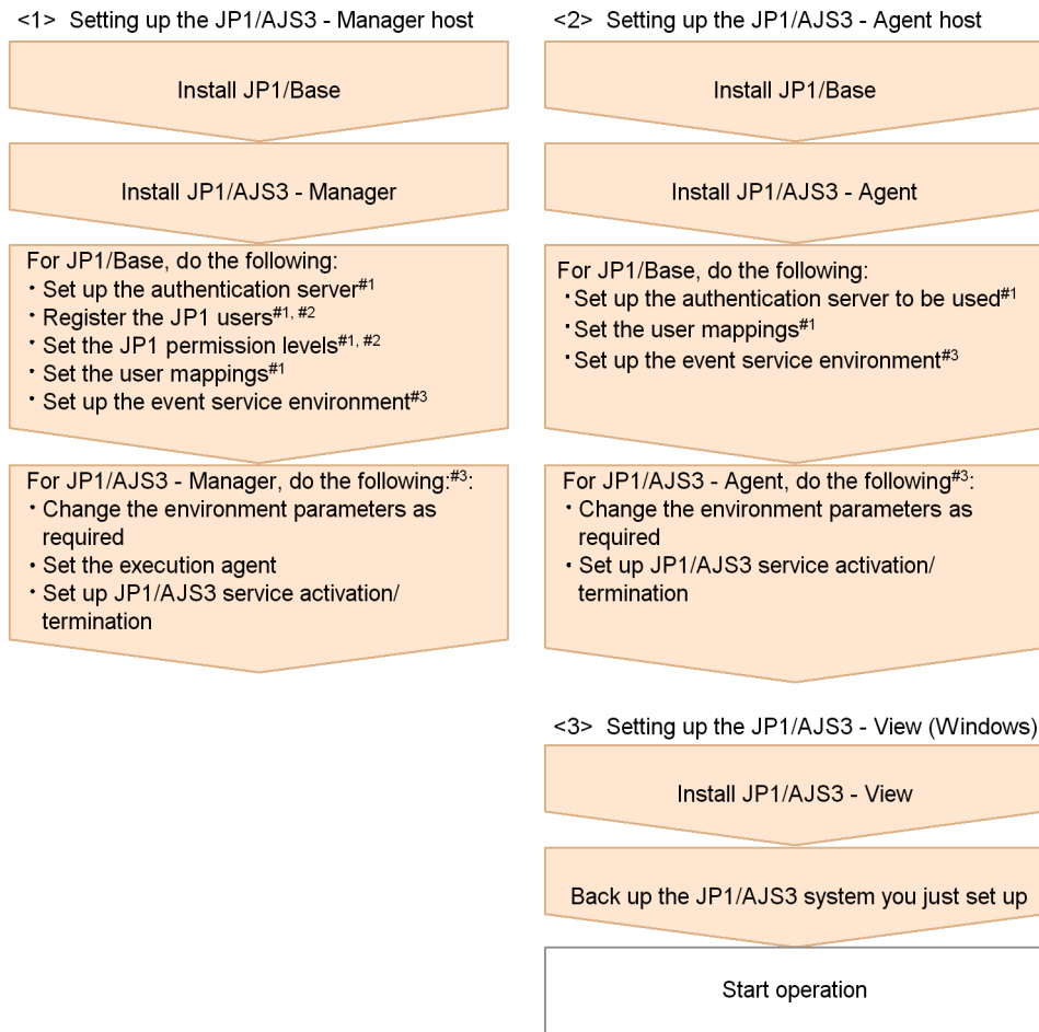
Figure 10-2: Procedure for setting up a system in a manager/agent configuration that uses only one JP1/AJS3 - Manager host
