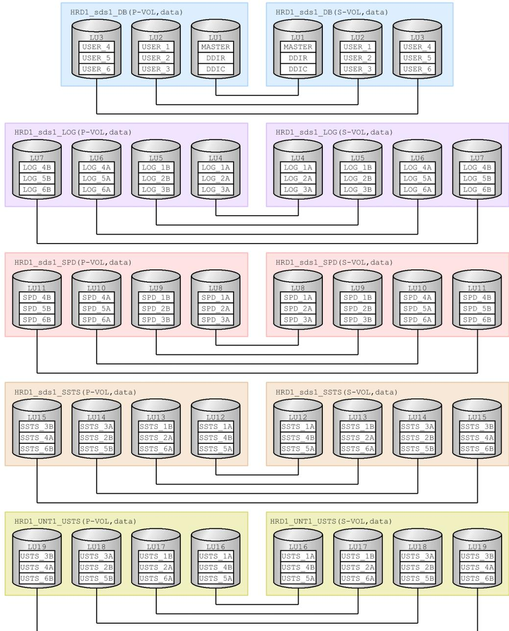
Figure 2-3: Paired volume configuration example (all asynchronous method)
