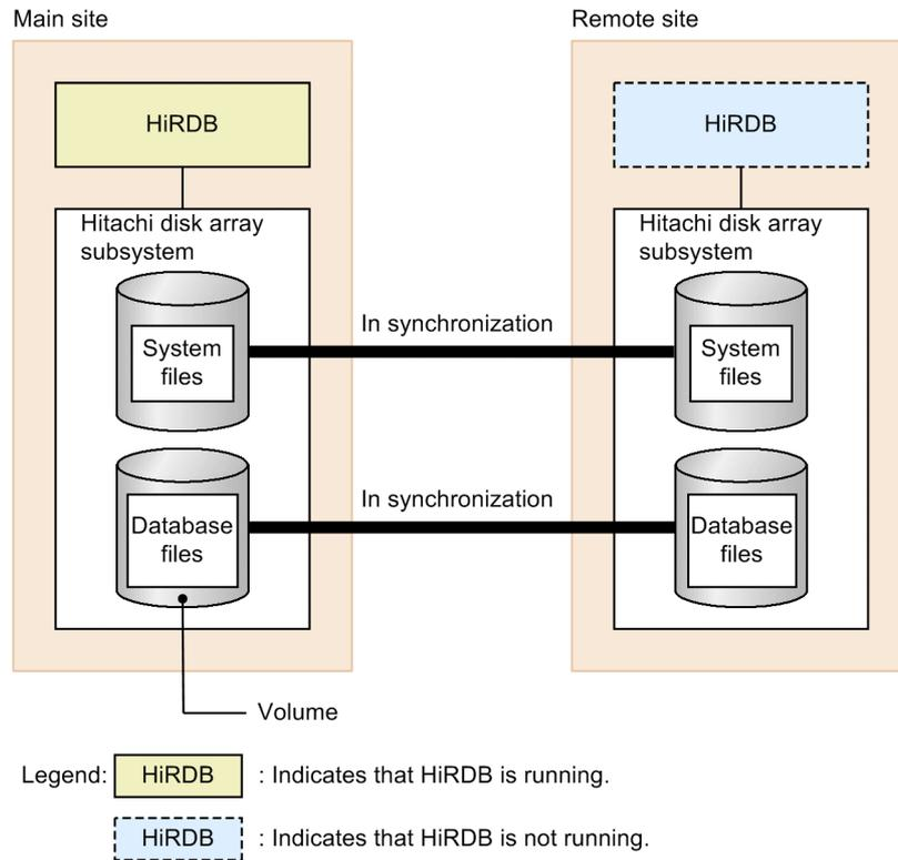
Table 1-2: Processing method used for update copying to the remote site (using the all synchronous method)
