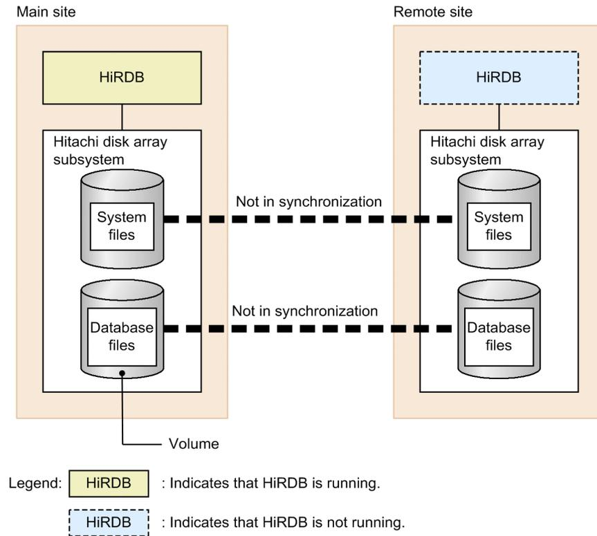
Table 1-3: Processing method used for update copying to the remote site (using the all asynchronous method)
