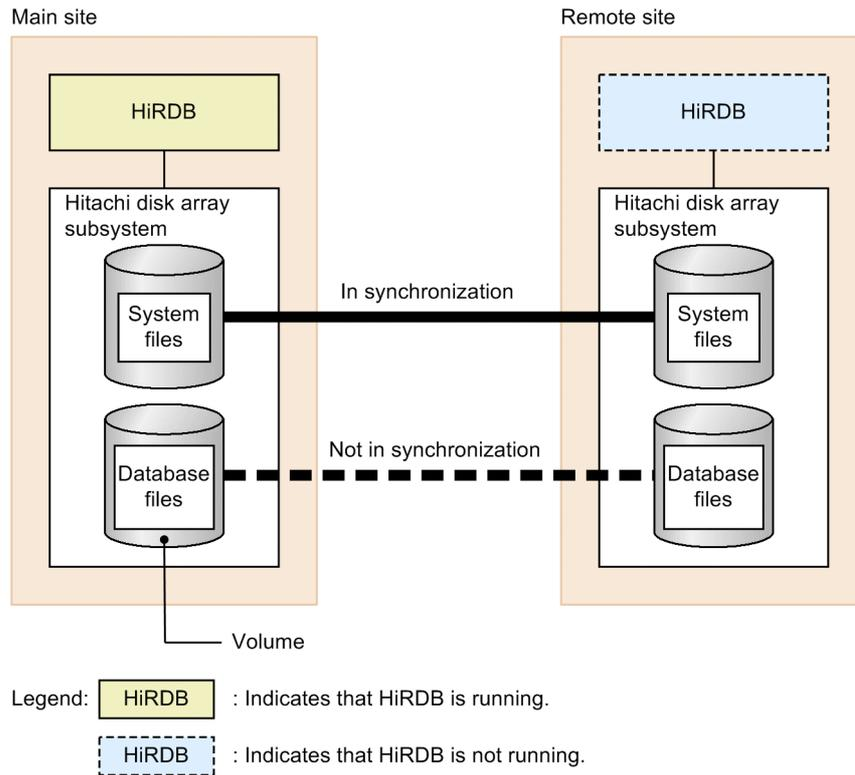
Table 1-4: Processing method used for update copying to the remote site (using the hybrid method)
