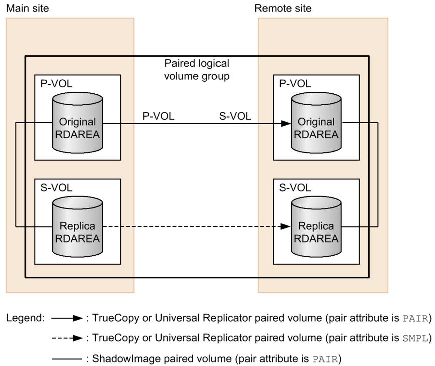
Figure 8-2: Pair volume configuration when the disks are not joined
