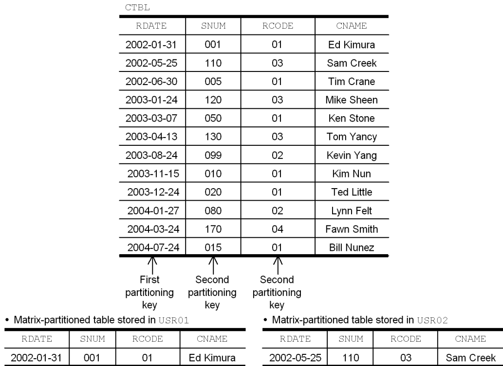
Figure 3-16: Example of matrix partitioning (combination of key range partitioning with boundary values specified and hash partitioning)
