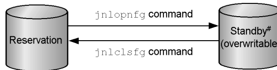
Figure 4-7: Status changes caused by open and close commands (system journal file)
